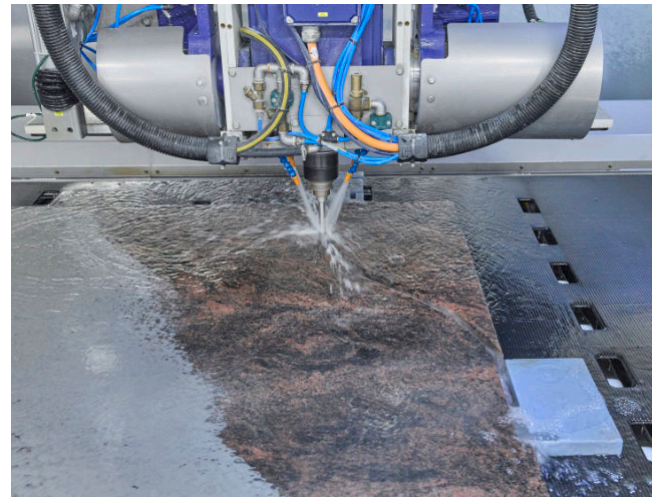
Above: The saw becomes a milling machine – machining of a curved cover plate.
