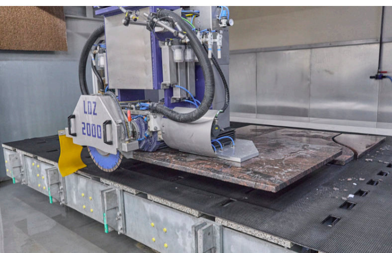
Thanks to vacuum separation, the saw saves valuable working time.
