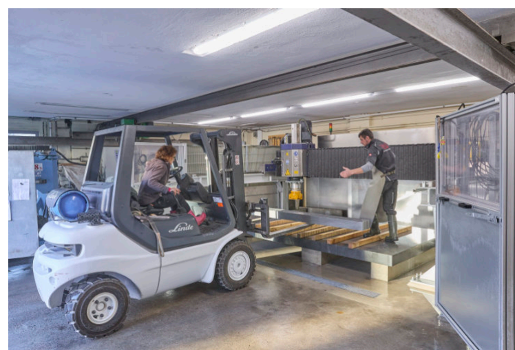
The surface grinding machine FSA 561 provides independence from material deliveries and offers many processing options.
