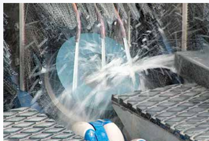
Unterfasssupport Lower chamfering head
